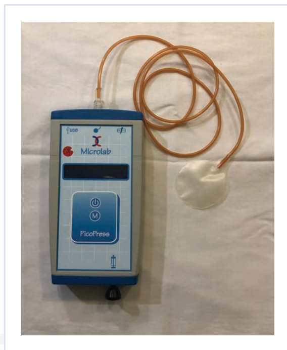
Fig 4. Example of a devices used to measure interface pressure in vivo , PicoPress
